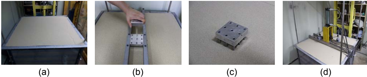
Figure 3 Procedure for axial load tests : (a) Making the model specimen; (b) Installation of micropiles; (c) Completion of group micropile; and (d) Performance of axial load tests
